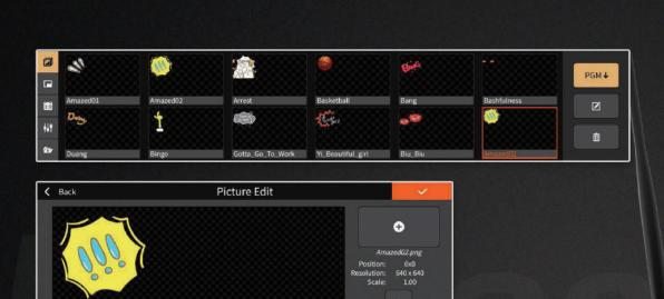
NSCaster X1's 4G bonding version of CG panel can publish pictures to the PGM monitor interface. It has built-in a large number of picture material and support importing external png/jpg format pictures. It also can move the position of the picture and the same channel can supports up to 12 pictures.
