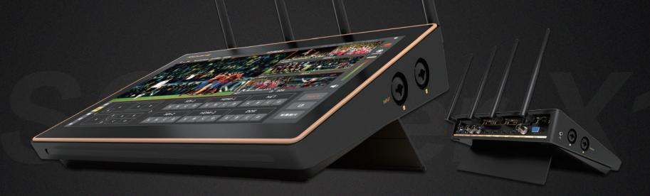
NSCaster X1 4G bonding version is a highly integrated navigation tablet with a built-in 11.6-inch full HD touchscreen monitor. It integrates functions such as multi-channel switching, recording, broadcasting, audio mixer, special effects, and monitoring. It also has built-in Ethernet, WIFI, and 4G bonding modules to meet the needs of webcasts for different scenarios.
